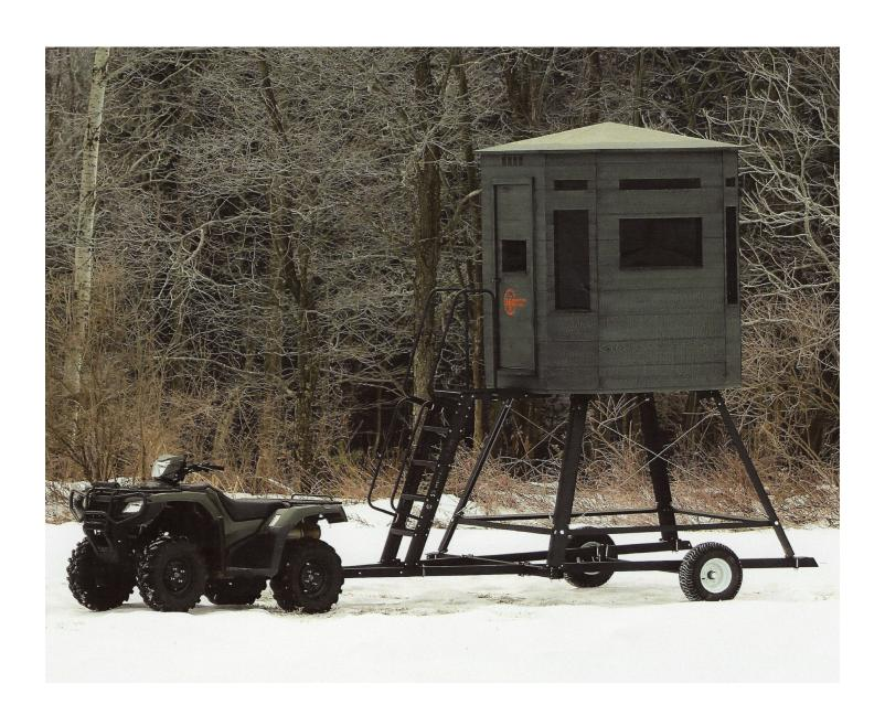
When relocating trailer, install jacks on top of cross bar and move slowly and cautiously.
